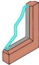
3D sketch of the window with two panes of glass
