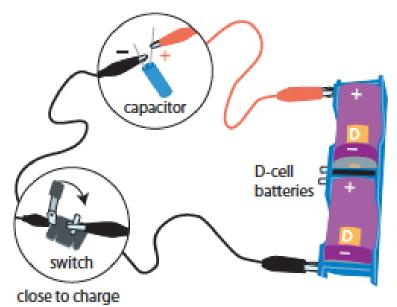
Identify the + and – wire leads on the capacitor. The + lead is longer. Connect – to – and + to +. Make sure that the the metal clips are not touching each other during charging or discharging.
