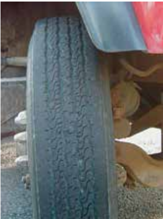
Driving on a worn-out tire is dangerous because there isn't enough friction between it and the road.
