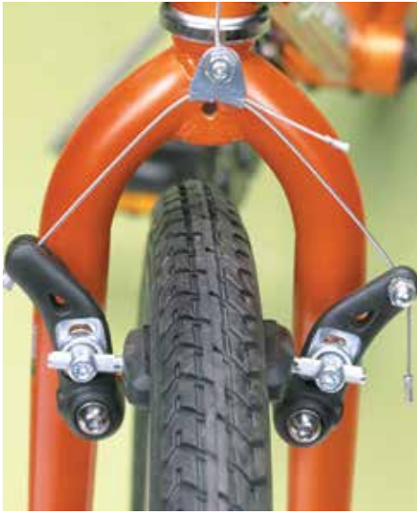
A bicycle brake, above, uses friction between the brake pads and the wheel rim to stop or slow down. In the photo on the right, a mechanic inspects a brake. If the parts become too worn, they won't generate enough friction to stop the car quickly.
