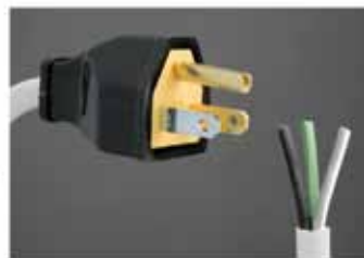
A three-pronged, polarized plug where the brass shows the hot line, the silver shows the neutral line, and the grounded prong is U-shaped. The wires also show hot (black), ground (green), and neutral (white) lines.
