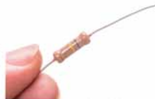
The value of the resistance on an electrical resistor can be identified by the colored stripes on it.
